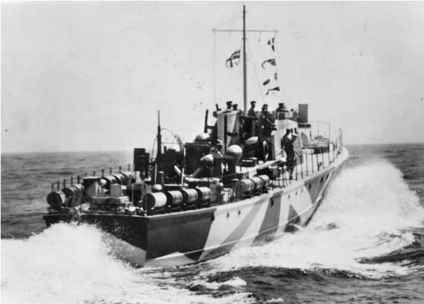
**RAN Fairmile motor launch ML 814 at speed. The depth charges seen aft were not carried on Operation *Adder***
