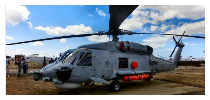
The Seahawk's main weapon is the MK 46 torpedo and it can also be fitted with a 7.62 mm door mounted general purpose machine gun. It is also used in search and rescue, troop lift and tactical insertion, utility operations (winching and external load lift) and fire bombing.
