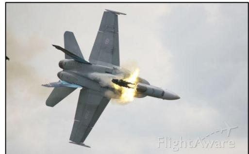
In the third photo (below) you can see the brain in the seat taking over, it realizes that leaving the aircraft and heading off parallel to the ground is not the ideal way to do things, so it changes the thrust of the rockets and sends the seat vertical to the ground, giving the pilot more height before he and seat part company and the pilot's parachute opens.
