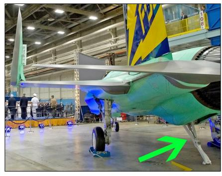
simply attach a longer hook to it in order to fix the problem as it has to fit inside the aircraft itself or the jet's low observable design will be compromised.
