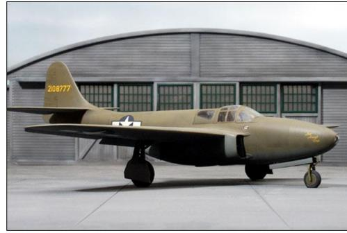
nacelles integrated within the main fuselage.
