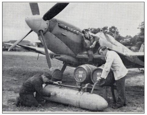
As a result, Spitfires equipped with Mod XXX or keg-carrying pylons were often sent back to Great-Britain for "maintenance" or "liaison" duties. They would then return to Normandy with full beer kegs fitted under the wings.
