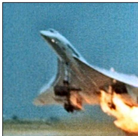
Shocking evidence now emerging suggests that the Air France Concorde F-BTSC had not been properly maintained. The airline's ground staff had failed to replace a "spacer" — a vital component of the landing gear which keeps the wheels in proper alignment. Although the BEA disputes it, there is compelling evidence that it was the missing spacer which may have caused the plane to skew to the left, so forcing Marty to leave the ground too early.
