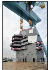
Nimitz-class carriers. It will be equipped with a new multi-band, multi-function radar and an island that is shorter in length and 20 feet (6.1m) taller than that of the *Nimitz*-class. The Island is set 140 feet (43m) further aft and 3 feet (0.91m) closer to the edge of the ship which will allow an increased launch rate for the 75 plus aircraft that will live aboard the carrier.
