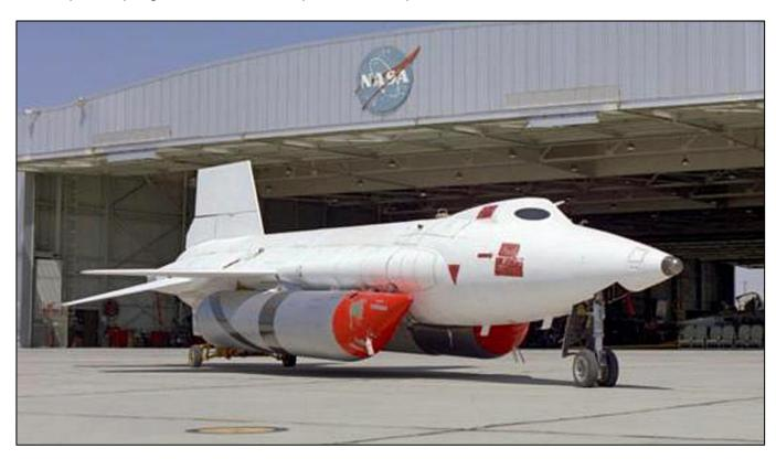
The record setting X-15A-2, aircraft number 56-6671, with its unusual white heat resistant ablative coating and giant anhydrous ammonia tanks under its fuselage.
