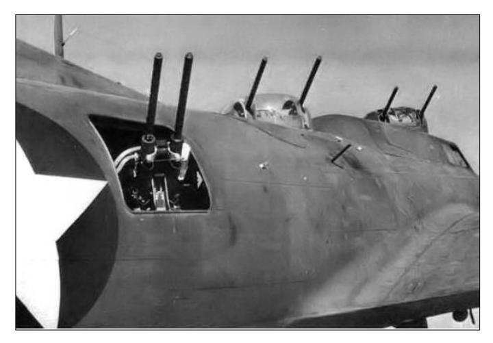
Work on the prototype began in September, 1942. The aircraft differed from the standard B-17 in that a second manned dorsal turret was installed in the former radio compartment, just behind the bomb bay and forward of the ventral ball turret's location. The single .50-calibre
