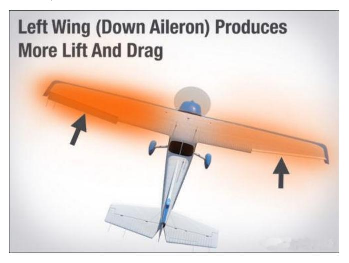
Try imagining the aileron as a miniature flap. When you lower flaps, your wings produce more lift and more drag. So when one of your two ailerons is lowered, the total lift and total drag acting on that wing increases, yawing the plane into that wing.
