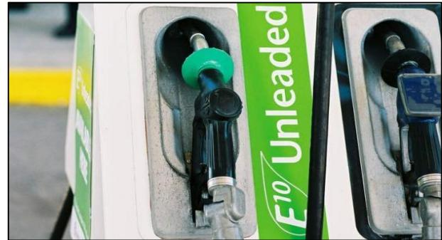
Most modern cars (those with fuel injection instead of carburetors) can use E10. You can check if your car is capable of running on E10 by consulting the owner's manual. Alternatively, many new cars will have a sticker inside the fuel flap that tells you what fuel your car can run on, and whether it is compatible with E10. Alternatively, you can check [THIS](#) website which lists most cars and motor cycles and will advise whether or not you should use E10.
