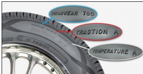
Traction is graded from highest to lowest as AA, A, B and C.
