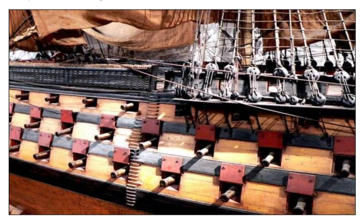
The lower, enclosed, gun deck usually mounted 32 pounders (15 cm calibre) while the upper gun deck, which was partially open to the elements, mounted 24 pounders. As each gun
