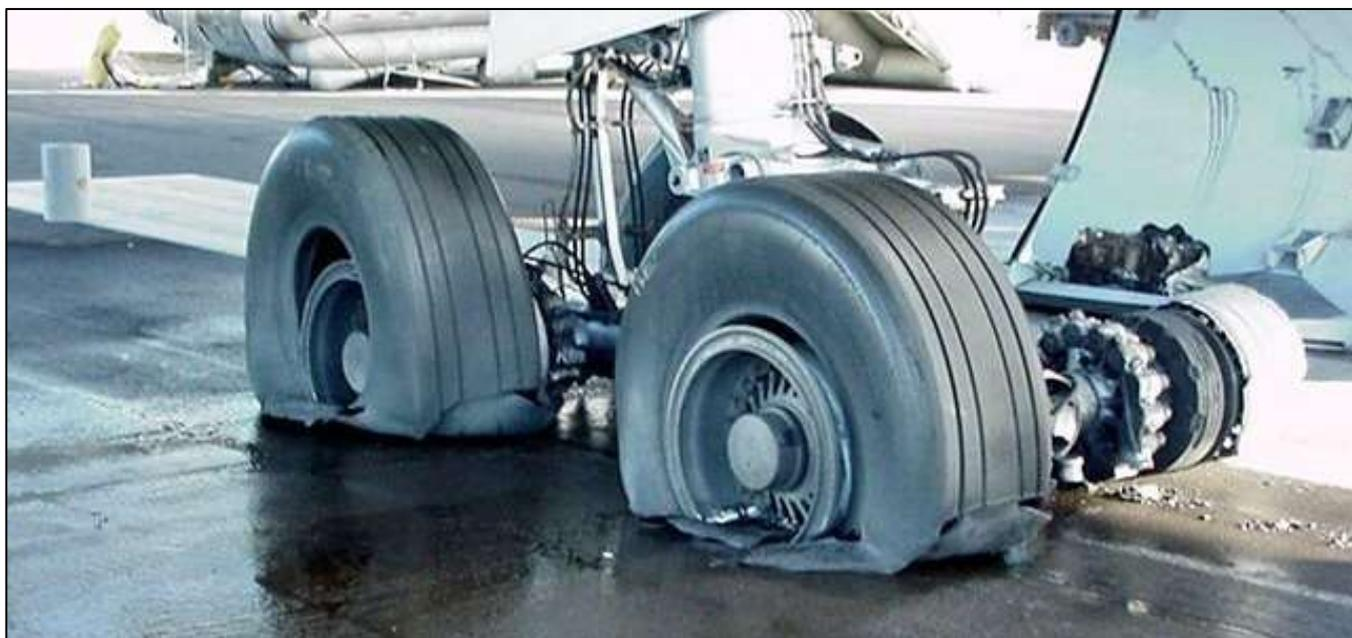
Fourteen passengers and two crew members suffered minor injuries, while two passengers suffered serious injuries during the evacuation of the aircraft. The plane suffered structural damage to the main landing gear and the lower fuselage.
