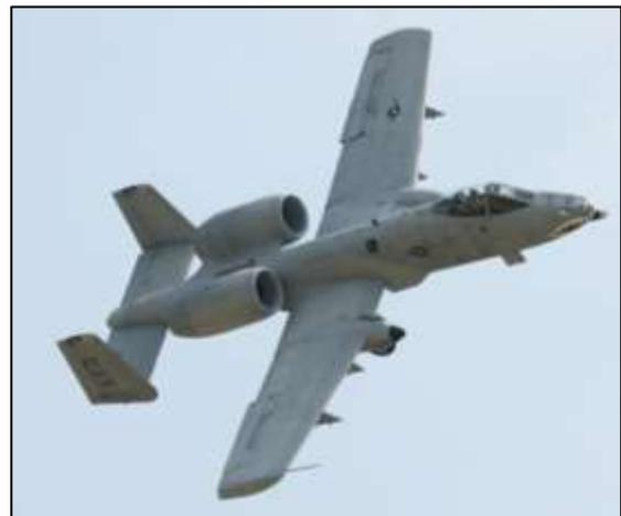
They were smart enough to make every part the same whether mounted on the left side or right side of the plane, like landing gear, for instance. Because the engines are mounted so high (away from ground debris) and the landing gear uses such low-pressure tyres, it can operate from a damaged airport, interstate highway, ploughed field, or dirt road.
