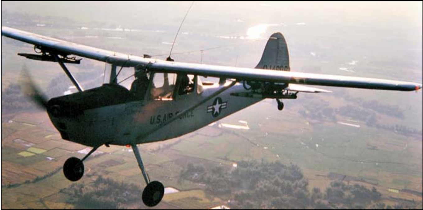
A Cessna O-1 'Bird Dog' fitted with four marking rockets. Photo by USAF FAC Gary Dikkers. The Bird Dog was developed from the Cessna 170.
