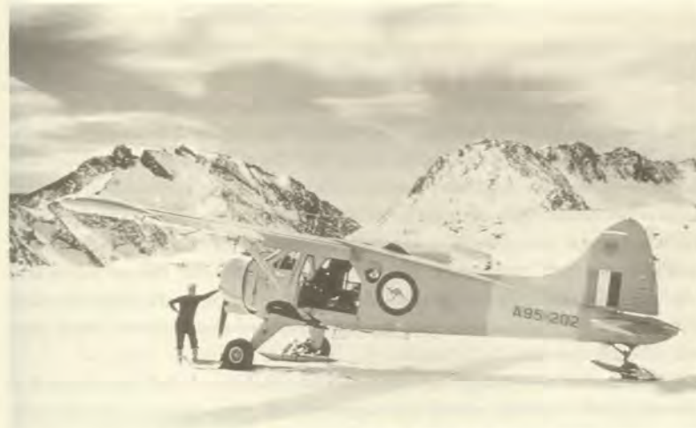
A95-202 poses against a backdrop of nunataks. Note the ski undercarriage, wide access doors and cameras mounted aft of access door. (RAAF Museum)
