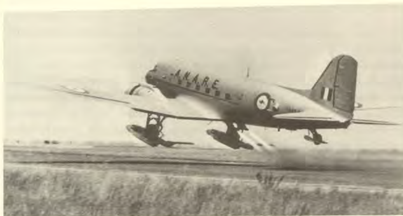
A65-81 undergoing JATO trials at ARDU. Note the skis and the camera mounts to the rear of the fuselage. (RAAF Museum)
