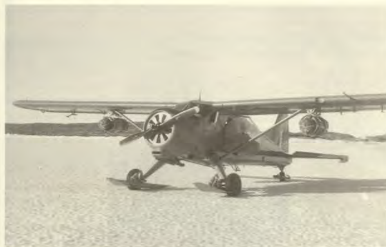
The Beaver, fitted with 25 gallon drums of diesel fuel on light series bomb carriers, is prepared to undertake a delivery. (RAAF Official)
