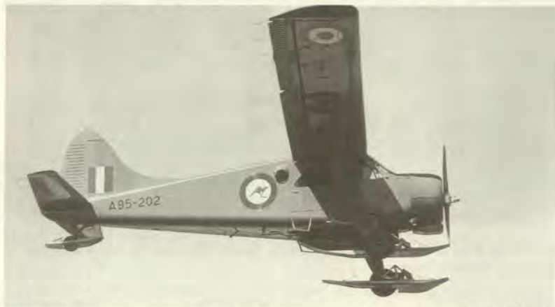
A95-202 shows her ski undercarriage and photographic equipment. (Dept. of Defence Public Relations)
