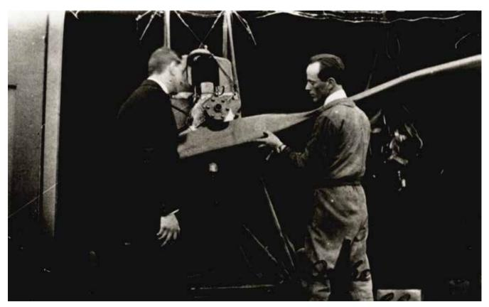
1913: Henry Chester (at right) fitting the propeller to the Deperdussin engine prior to engine tests at Victoria Barracks, Melbourne (RAAF Museum)
