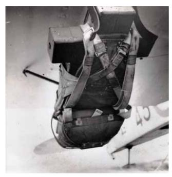
1926: wooden torso dummy for parachute testing mounted under the wing of a D.H.9 aircraft (RAAF Museum)
