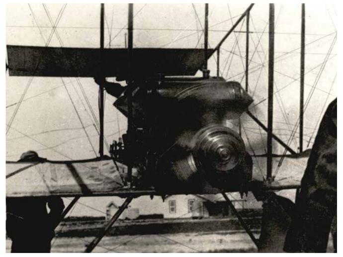
1915: Gnome engine of CFS8 clearly showing the rotary type construction with the cylinders attached to the propeller and stationary crankshaft (RAAF Museum)
