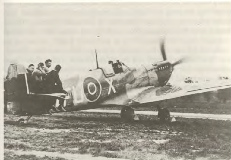
Groundcrew hold down the tail of Spitfire BS400 FU-X for an engine ground run.
