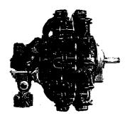
Pratt & Whitney R-1830 Twin wasp 14 cylinder Radial Piston Engine 1200 horse power.
