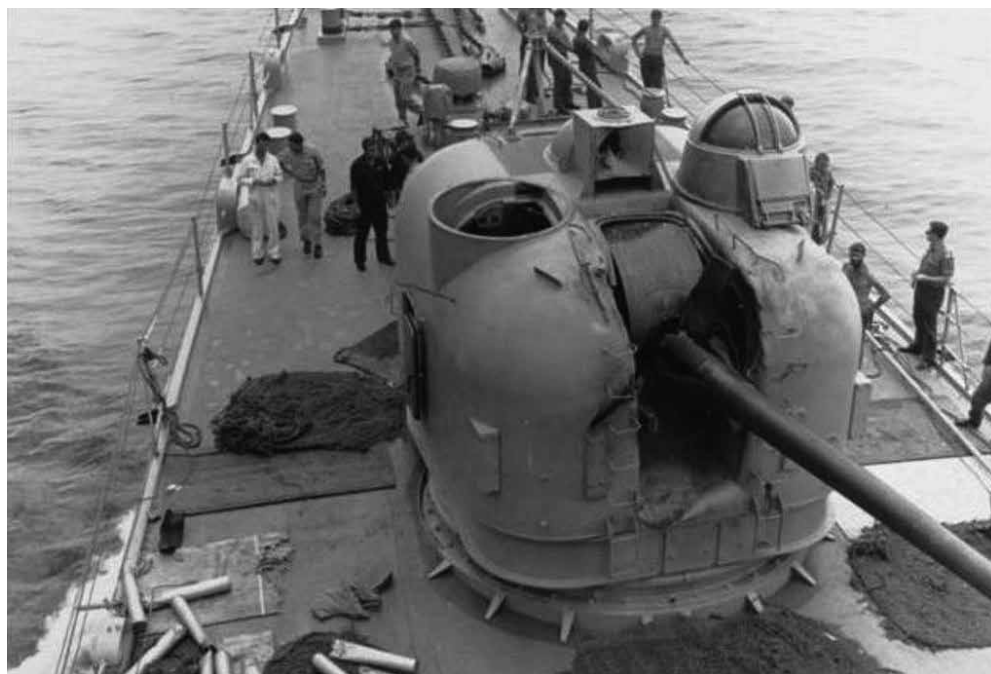
Damage to HMAS Brisbane 's forward 5-inch gun, off Vietnam, 22 July 1969 (Source: Rosey Kendall)
