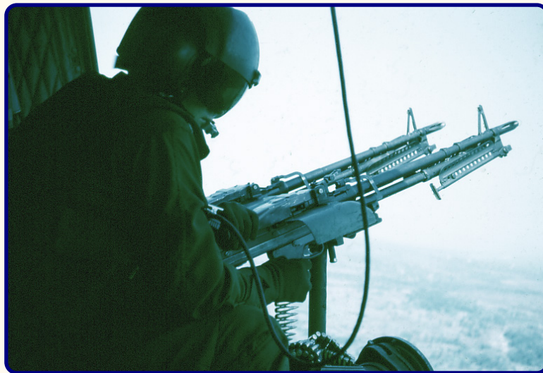
Port twin door-gun airstream deflectors (Image: Roger Buck)
