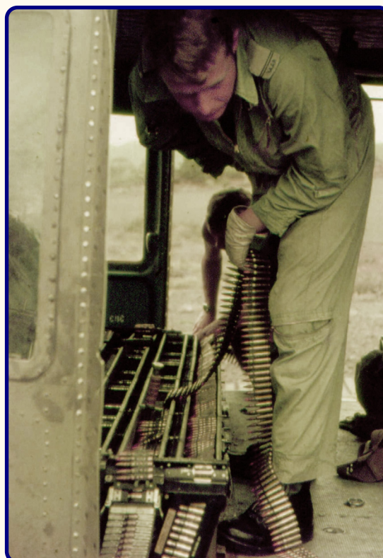
Loading the extended XM21 minigun ammunition stowage (Three images: Trevor Ward)
