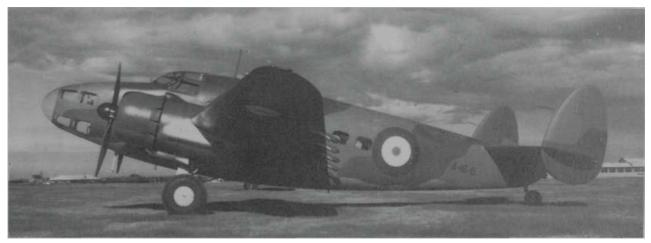
A16-6, one of the first Hudsons delivered to No 2 Squadron in June 1940, shows the lack of dorsal gun turret when these aircraft were originally delivered to the RAAF. F JEFFERIES
