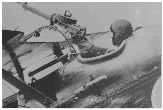
The overwing Lewis gun fitted to the SE-5A
