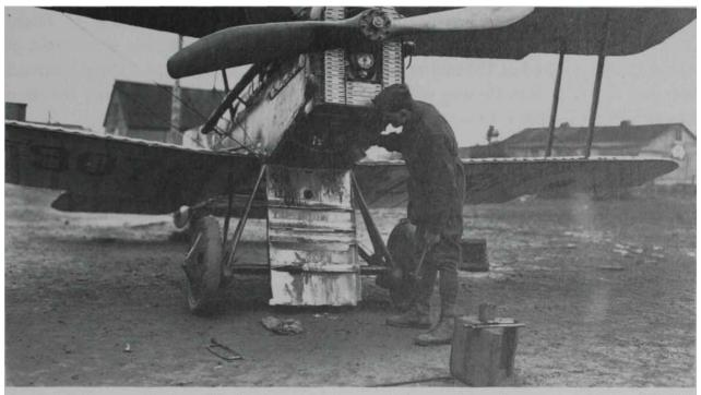
An Australian mechanic with the lower engine cowl dropped to allow access to the SE-5A's Wolseley engine AWM D439
