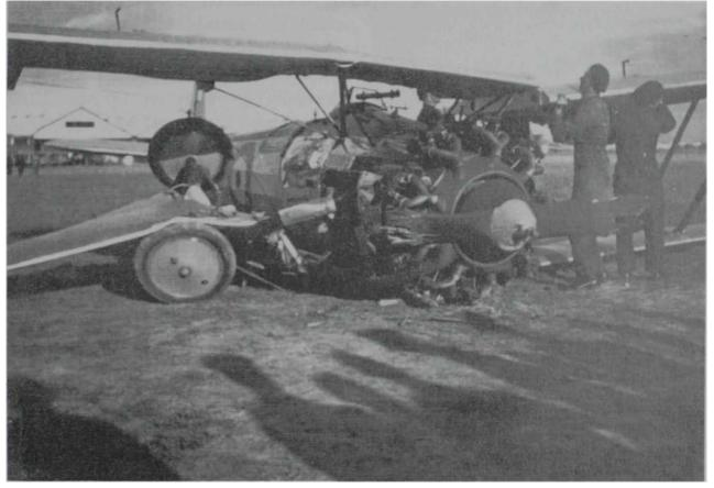
Although this hard landing for Bulldog A12-6 at Laverton on 2 April 193S looks like the aircraft was a write-off, it was repaired and returned to No 2 Squadron ivithin three months. VIA E PERKINS
