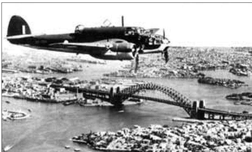
A9-700 – The Last Beaufort Delivered to the RAAF With D/F loop extended
