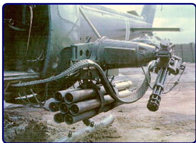
US Army Charlie model gunship with XM-21 System encompassing flex miniguns and remote fire control and aiming system fitted to left hand pilot station – Images: US Army
