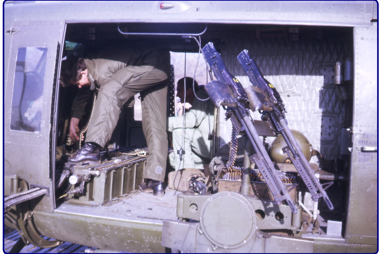
Reloading the extended XM-21 minigun ammunition stowage Images: Peter Robinson & Roger Buck
