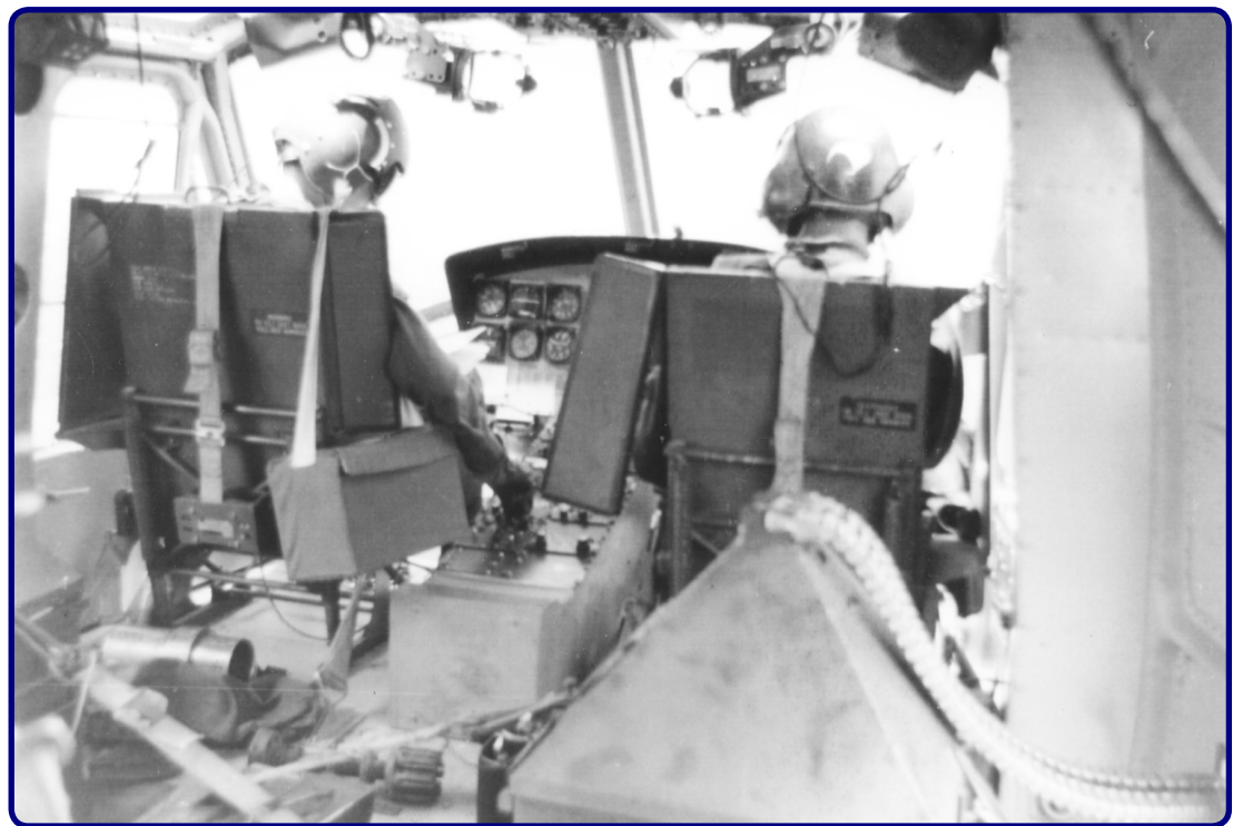
95QN improved minigun hopper ammunition stowage Images: Norm Goodall
