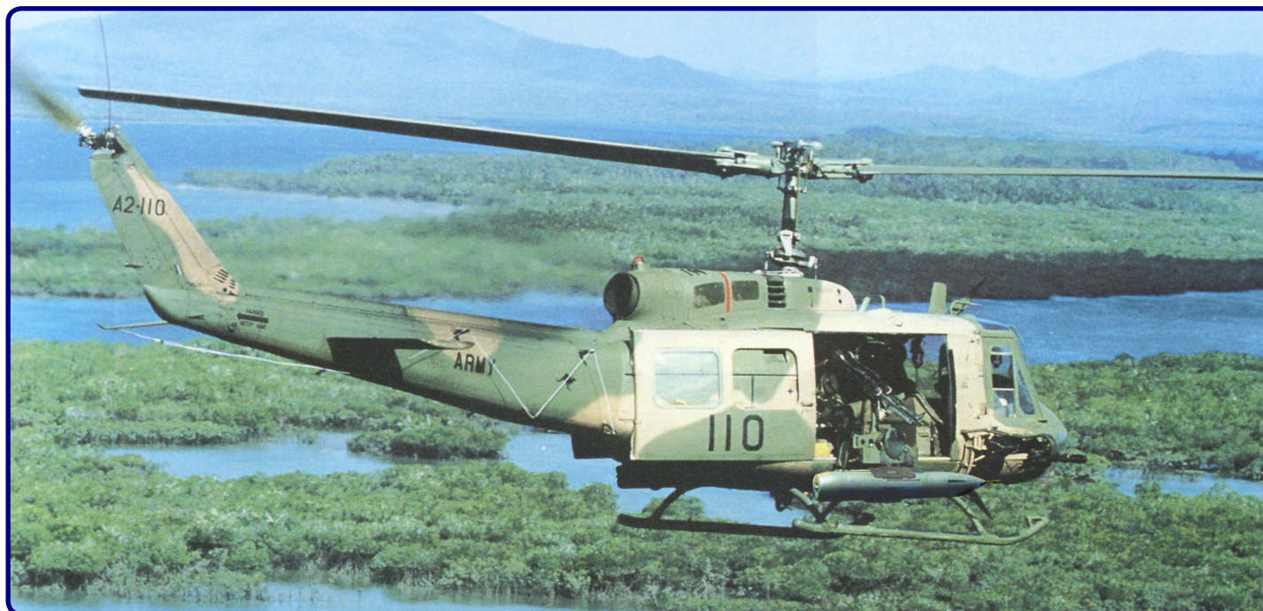
Conceptual ADF Huey II Gunship – Primary Image: Australian Army 2 x NC621 podded low recoil 20mm cannon substituted for 70mm rocket launchers
