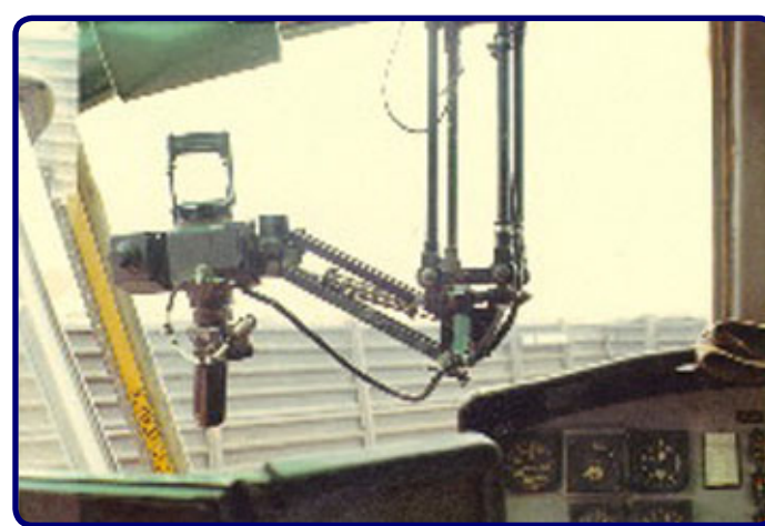
US Army Charlie model gunship with XM-21 System encompassing flex miniguns and remote fire control and aiming system fitted to left hand pilot station – Images: US Army
