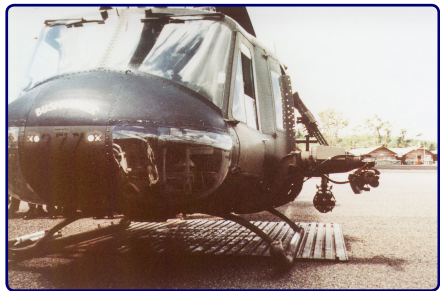
Changed XM-21 System configuration showing rocket launcher harmonization clearance Image: Air Force
