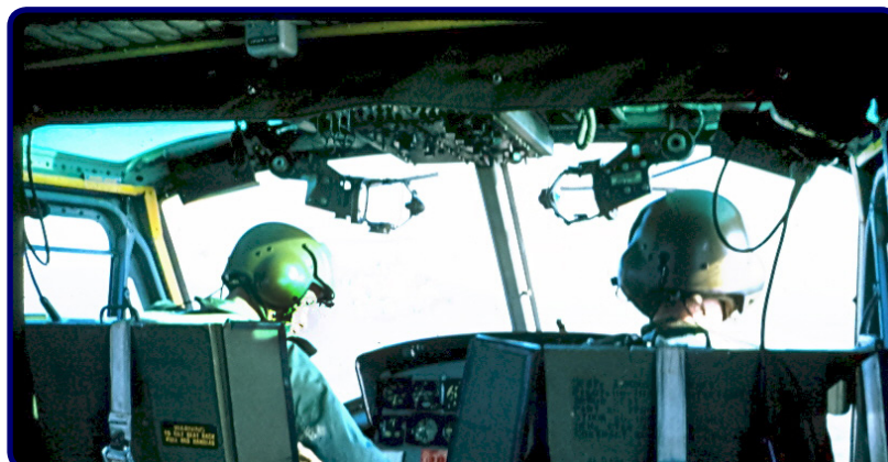
Standard single US Army right hand gunsight and twin sights adaptation for Hotel model Images: 9SQN Gunship Project & Terry Pinkerton
