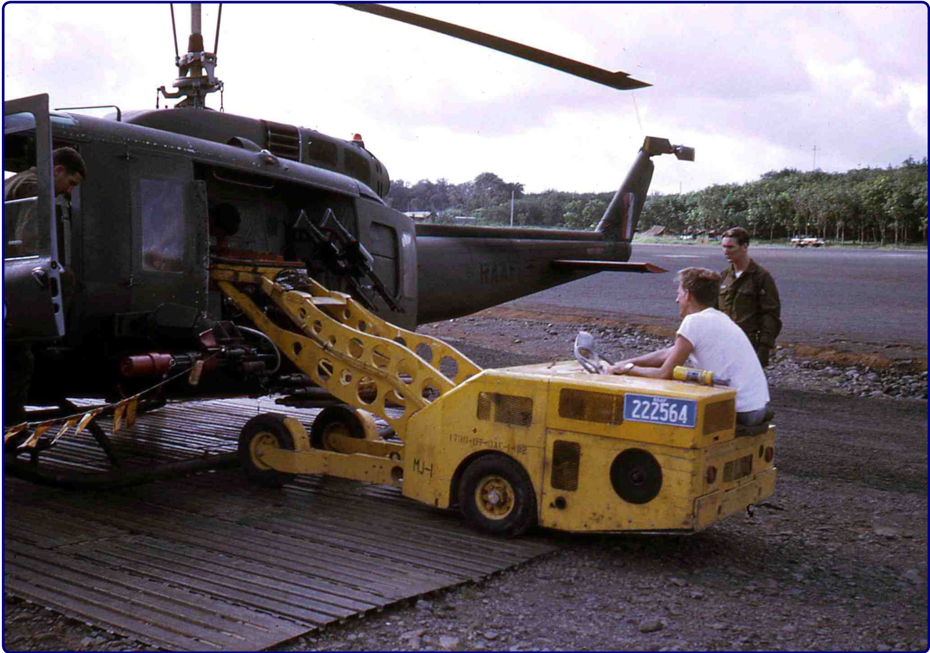
Reloading minigun hopper ammunition bins – Images: Norm Goodall
