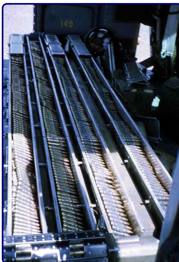
Extended XM-21 System minigun ammunition stowage, capacity 9,600 rounds Image: Norm Goodall
