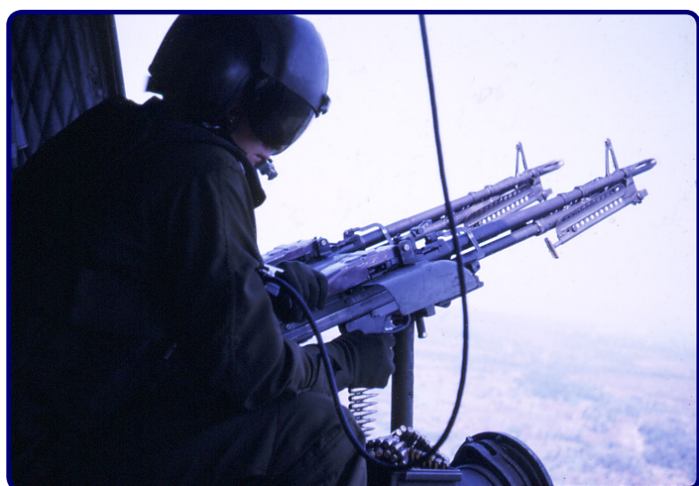
Port doorguns airstream deflectors and starboard doorguns ammunition feeds Images: Roger Buck & Terry Pinkerton
