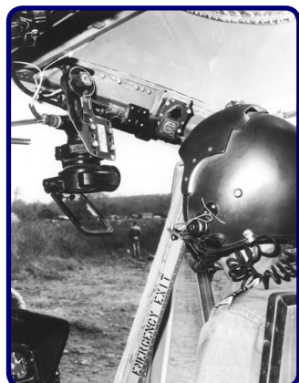
Standard single US Army right hand gunsight and twin sights adaptation for Hotel model Images: 9SQN Gunship Project & Terry Pinkerton
