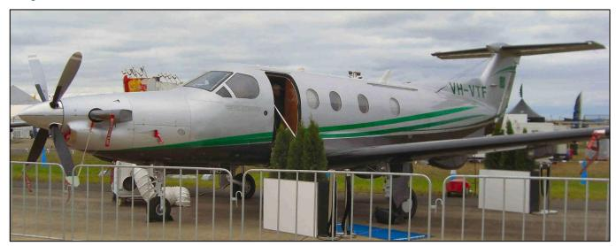
Unlike the Cessna, the Pilatus is pressurised and cleans up in flight. Cruise speed is 500Klm/hour at 20,000ft, giving a range of 2,800 klms fully loaded and following recent
