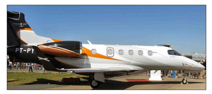
The Phenom can carry 8 or 9 occupants with a flying range of 1,971 nautical miles and you can have a new one for only \$8M. It's a pressurized aircraft and at 45,000 feet, it has a cabin altitude of 6,000 feet.
