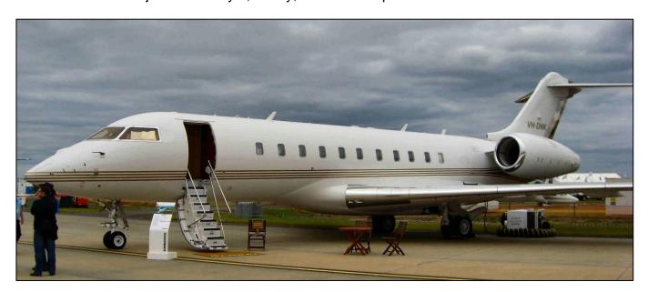
The Bombardier is an ultra long-range corporate and VIP high speed jet aircraft and is powered by two BMW Rolls Royce BR-710 turbofans. It can fly up to 19 passengers, in sumptuous comfort, intercontinental ranges without refueling as its typical range is 6,325 nm (11,400 klm) at a cruise of 488 kt (900Klm/h) with a service ceiling of 51,000 ft.
