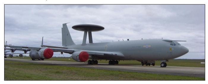
It can cruise at 400 kts at 30,000ft and can scan at distances over 300nm, it can detect low-flying targets or maritime surface contacts within 215nm and it can detect medium-level airborne targets at ranges in excess of 280nm.
