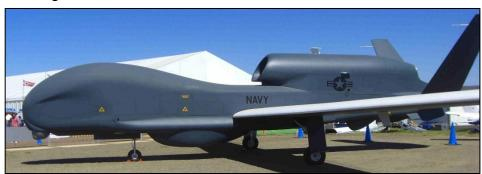
It is able to provide high resolution radar that can penetrate cloud-cover and sandstorms and Electro-Optical/Infrared imagery at long range with long loiter times over target areas. It can survey as much as 40,000 square miles (100,000 square klms) of terrain a day. They cost about \$35 million each.
