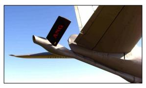
refueling, the large flyable boom attached to the airplane's belly can offload fuel at the rate of 6,500 pounds per minute. This is enough fuel in one minute to operate an average family car for one year.
