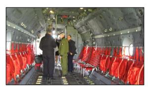
The Spartan is constructed with a floor strength equal to that of a C-130 and the large cargo cabin cross-section is able to accommodate Hercules pallets.
