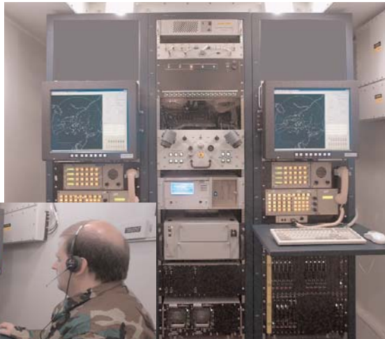
The AN/TPS-77's PMFL system continually monitors the radar status and reports system status to remote maintenance centers.
