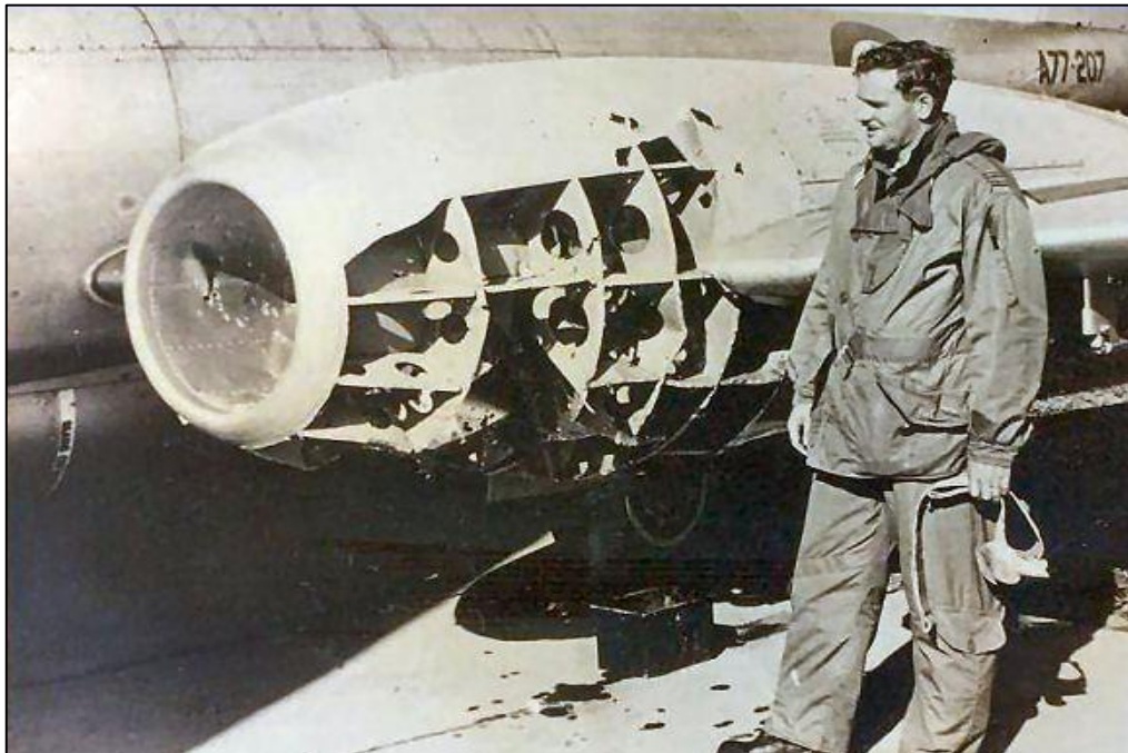
Jack McCarthy standing in front of Geoff's aircraft, A77-207, which suffered severe flack damage. The aircraft performed reasonably well on one engine.
