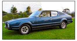
The Force 7 was one of the first hatchbacks to be released in Australia. There were to be three models of increasing price and luxury, from the base model equipped with a six cylinder engine and 3-speed column shift gearbox, followed by the awesome Force 7V fitted with a powerful 4.4 litre V8 'four-on-the-floor'. At the top of the tree was the "Tour de Force", featuring leather interior.
