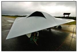
be the forerunner of the next generation of stealthy robot-strike aircraft. Its geometry and radar-absorbent materials make it difficult to impossible to spot on radar. Operating from aircraft carriers, the UCAS-D could fulfil the Navy's goal of an aircraft that can carry a payload (such as bombs) of up to 2,000 pounds, plus an extra 2,500 pounds externally when stealth is not required. A
