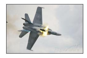
In the third photo (below) you can see the brain in the seat taking over, it realizes that leaving the aircraft and heading off parallel to the ground is not the ideal way to do things, so it changes the thrust of the rockets and sends the seat vertical to the ground, giving the pilot more height before he and seat part company and the pilot's parachute opens.
