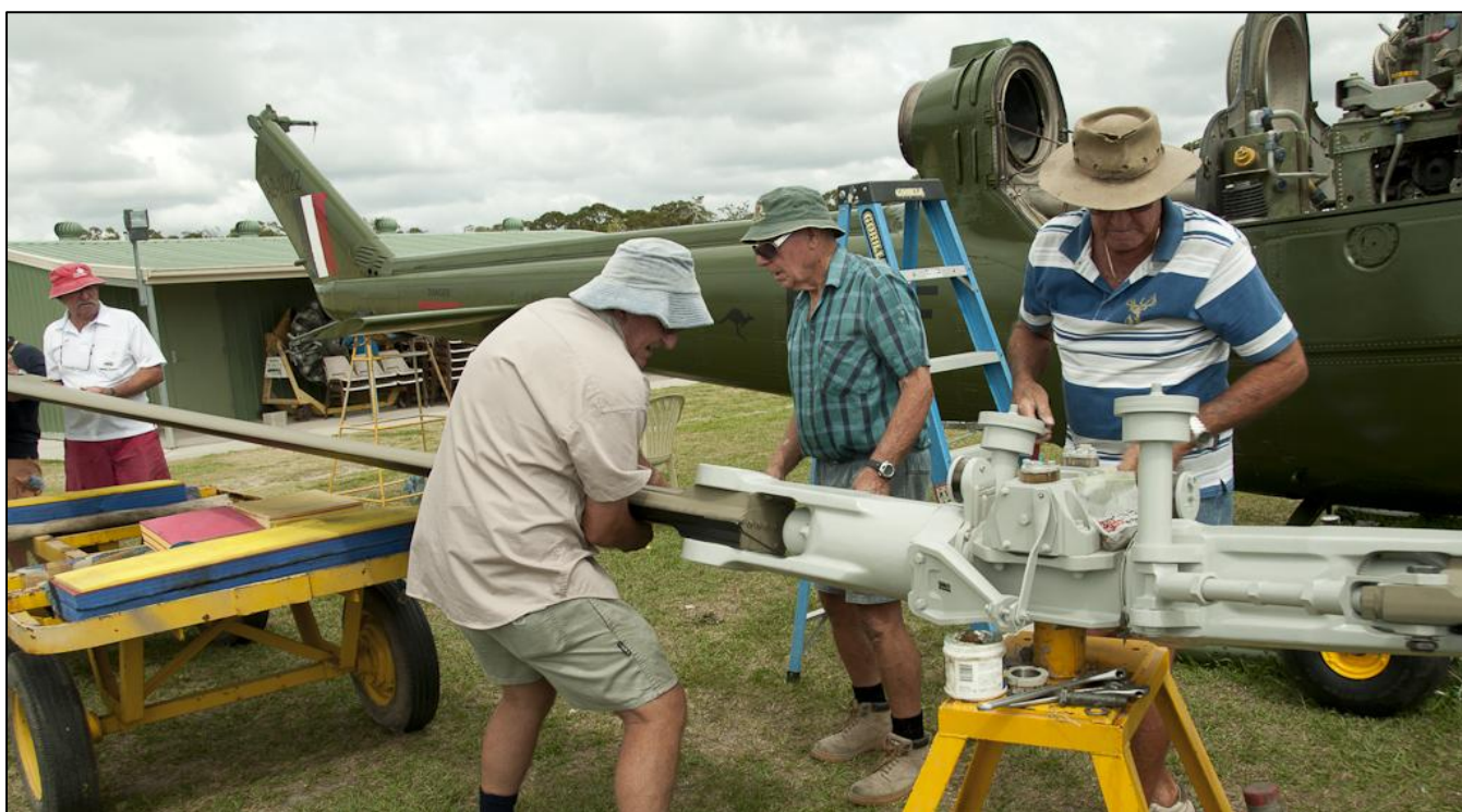
Working on the rotor are L-R: Way out left in the pink hat is Bob McInnes , then Ian Newham , a civvy, fitting the rotor into the blade grip, Bill Wiggett , ex Army Nasho in the green hat, Roy Robinson , ex RAAF metal basher.
