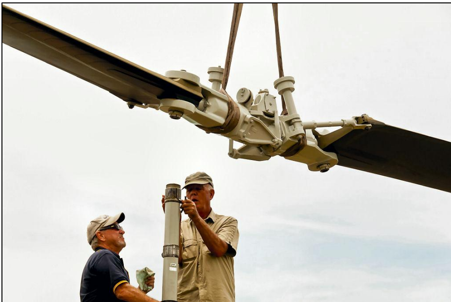
Kerry Millard and, Ingo Meier check the rotor mast prior to fitting the rotor.
