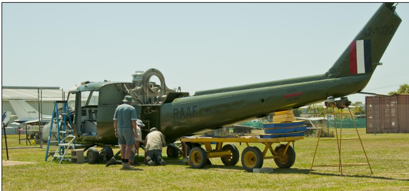
Fitting the tail boom to the rest of the balus are: L-R: Bill Wigget , Ian Newham and Ingo Meier kneeling – or is he praying??
