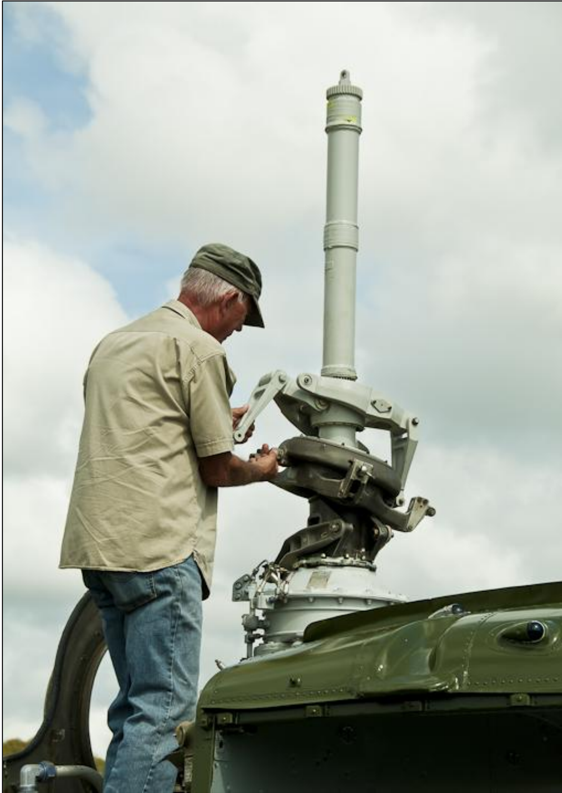
Ingo Meier ex appy Framie, then Engo, checking out the swash plate assembly prior to fitting the rotor.
