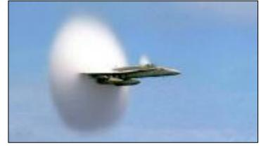
the air doesn't compress any faster than the speed of sound. But the energy has to go somewhere. It ends up making an area of high pressure around the airplane, a shock wave.
