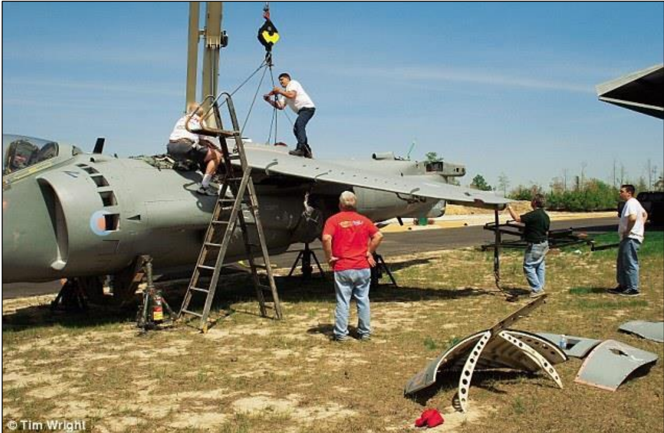
Attaching the wing after the plane's arrival in the U.S. in 2006.
