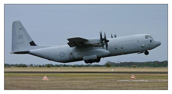
The C-130J is a comprehensive update of all previous models with new engines/props, flight deck, and other systems. Externally similar to earlier models, the J-model features considerably updated technology. These differences include new Rolls-Royce AE 2100 D3 turboprops with Dowty R391 composite scimitar propellers, digital avionics and reduced crew requirements. These changes have improved performance over its C-130E/H predecessors,
