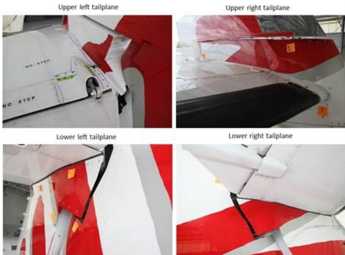
Figure 2: Tailplane external damage (indicated by marks and stickers)
