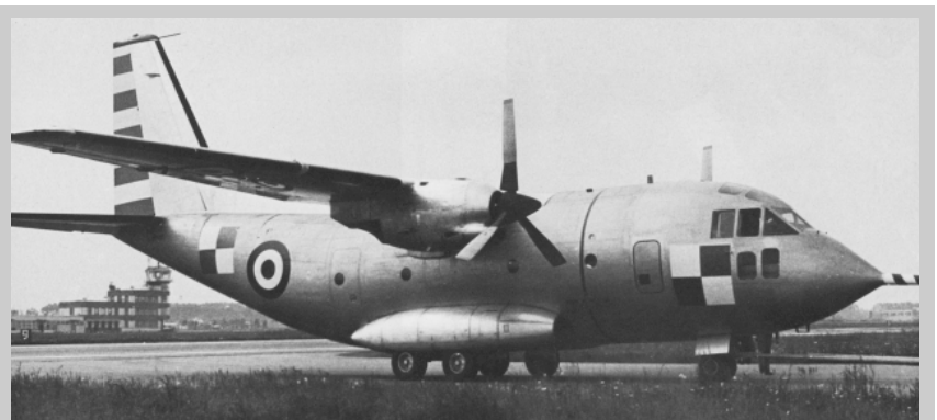
Above: Following a re-design, the Fiat G.222 prototype emerged in 1970 as a more conventional Short Take Off and Landing transport with a larger fuselage and wingspan.
