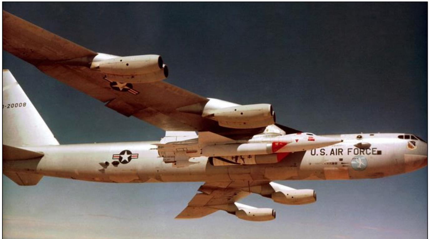
The X-15, slung beneath the B-52 – enroute to another record breaking flight.
