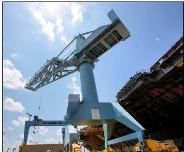
When you first see the ship in the dry-dock, it looks like it is being built from second-hand steel. Not so. This is done to save on repainting over welds and stresses caused during construction, painting is only done after the ship is complete. Raw steel exposed to salt air causes the rust, but the various other colours denote the
