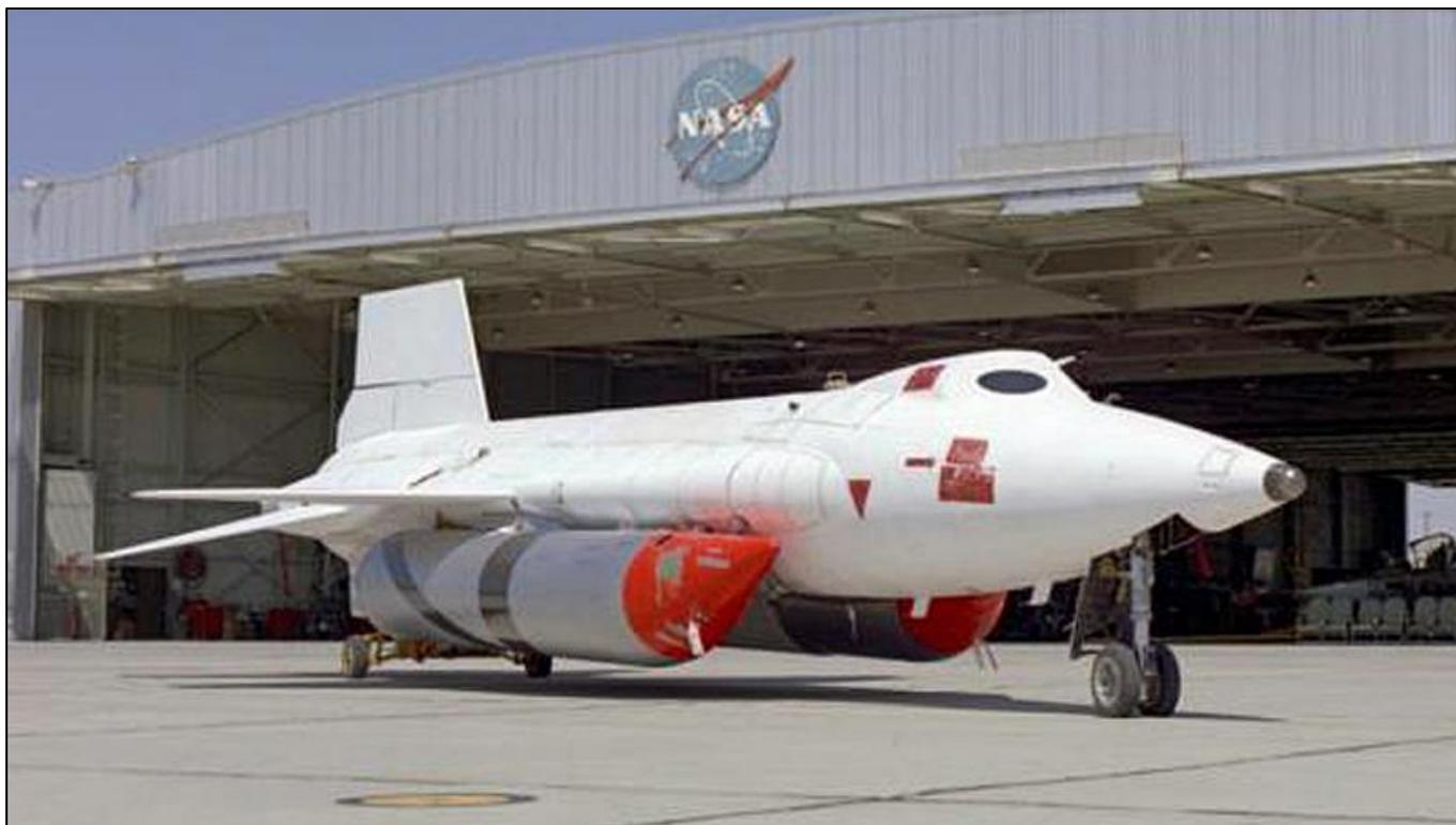
The record setting X-15A-2, aircraft number 56-6671, with its unusual white heat resistant ablative coating and giant anhydrous ammonia tanks under its fuselage.
