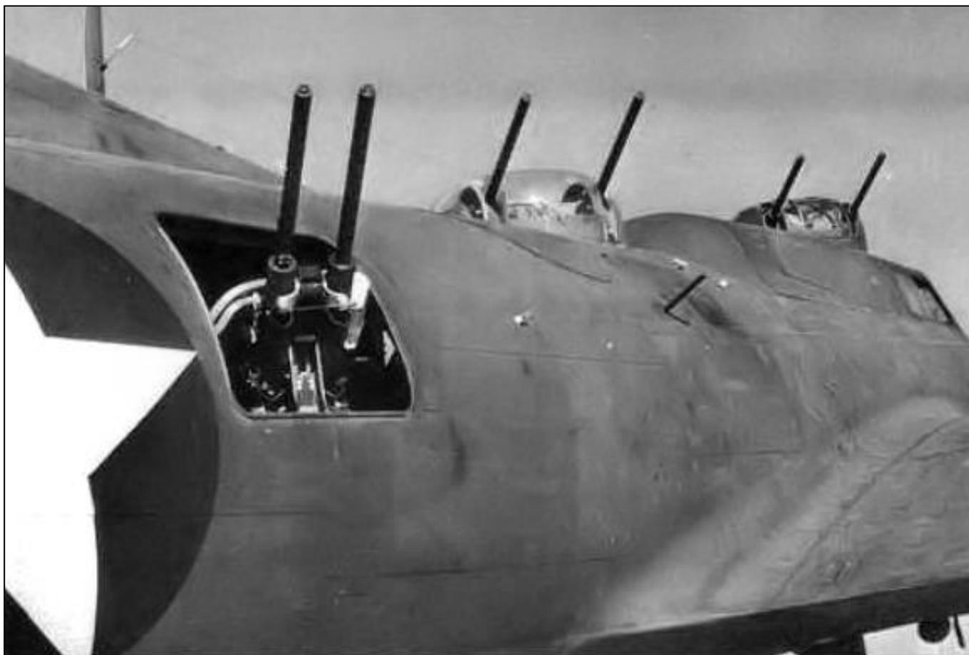
Work on the prototype began in September, 1942. The aircraft differed from the standard B-17 in that a second manned dorsal turret was installed in the former radio compartment, just behind the bomb bay and forward of the ventral ball turret's location. The single .50-calibre
