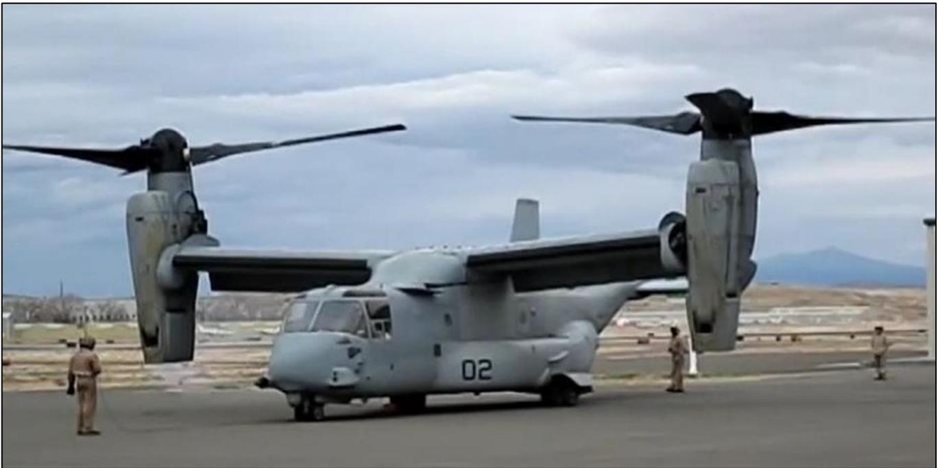
The Osprey is equipped with 16 fuel tanks (ten integrated into the wings and six in the fuselage), giving it a range of just under 900 nautical miles (1,700 klms) however, the aircraft is capable of being refuelled while airborne. Boeing is also developing a roll-on/roll-off aerial refuelling kit, which would give the V-22 the ability to refuel other aircraft.
