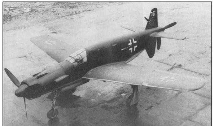
Claudius Dornier had patented the push-pull engine layout in 1937, which was innovative because it offered the power of two engines but less drag and greater manoeuvrability than other twin-engine configurations. The RLM (German Aviation Ministry) wanted to support development of push-pull aircraft but initially only as seaplanes and bombers. By 1942, the Luftwaffe needed multi-role fighters and after submitting a proposal in January 1943 for a
