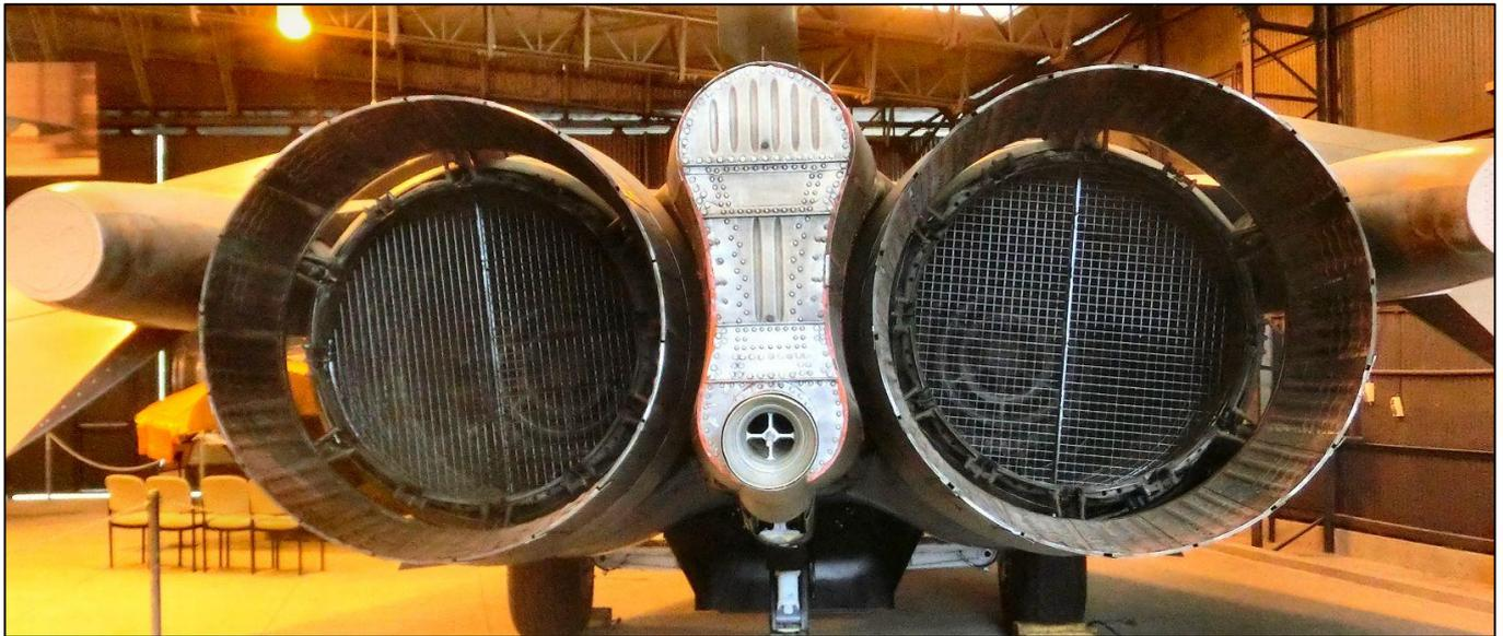
Most planes can dump fuel from their wings, however, the F-111's design put the dump nozzle in the back of the plane. This is the only reason these planes could do it, as when the fuel is dumped the pilot kicks in the afterburners and ignites the fuel.
