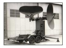
An interesting note. We techs would get a little bit peeved if the Air Traffic Os operating the system would consistently activate the "Precision" mode when the search antenna was a long way off alignment with the height finder antenna. As soon as activation occurred, the clutch would try to engage both antennae, but would have to wait until the next time the key slot came
