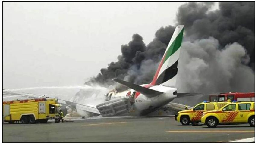
Secondly, a pilot colleague observed exactly what happened as he was there, waiting in his aircraft to cross runway 12L. The B777 bounced and began a go-around. The aircraft reached about 150 feet (45 metres) with its landing gear retracting, then began to sink to the runway. This suggests that the pilots had initiated a go-around as they had been trained to do and had practised hundreds of times in simulators, but the engines failed to respond in time to the pilot-commanded thrust. ... Why?
