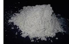
called magnesiothermic reduction, the group converted this low-cost source of Silicon Dioxide (SiO2) to pure silicon nano-particles.
