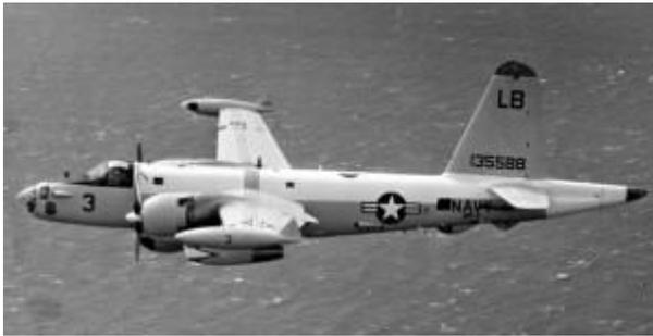
The Neptune was a twin-engine (with two small jet engines added in later models to increase takeoff performance) mid-wing aircraft with a crew of 10. Two pilots, navigator, tactical coordinator, flight engineer, radio operator, radar operator, two sensor operators, and an observer/mad operator. Neptunes were unpressurized so they normally stayed below 10,000' to avoid wearing oxygen
