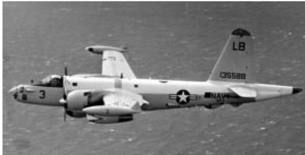
The Neptune was a twin-engine (with two small jet engines added in later models to increase takeoff performance) mid-wing aircraft with a crew of 10. Two pilots, navigator, tactical coordinator, flight engineer, radio operator, radar operator, two sensor operators, and an observer/mad operator. Neptunes were unpressurized so they normally stayed below 10,000' to avoid wearing oxygen
