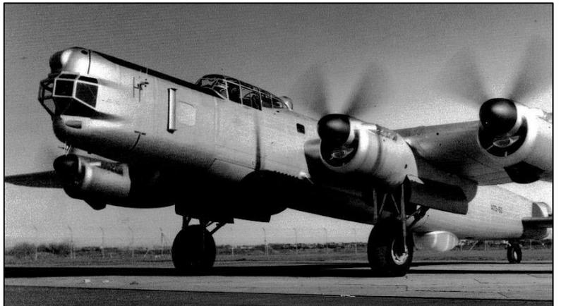
The picture of the Long Nose Lincoln above well illustrates why this aircraft was difficult to land especially at night in any crosswind. The long nose blocked the pilot's view of the runway as you flared for the landing and was worse when the tail was lowered during the landing run. Any crosswind made it worse. Initial part of the take-off run was a problem too, until you got the tail up.
