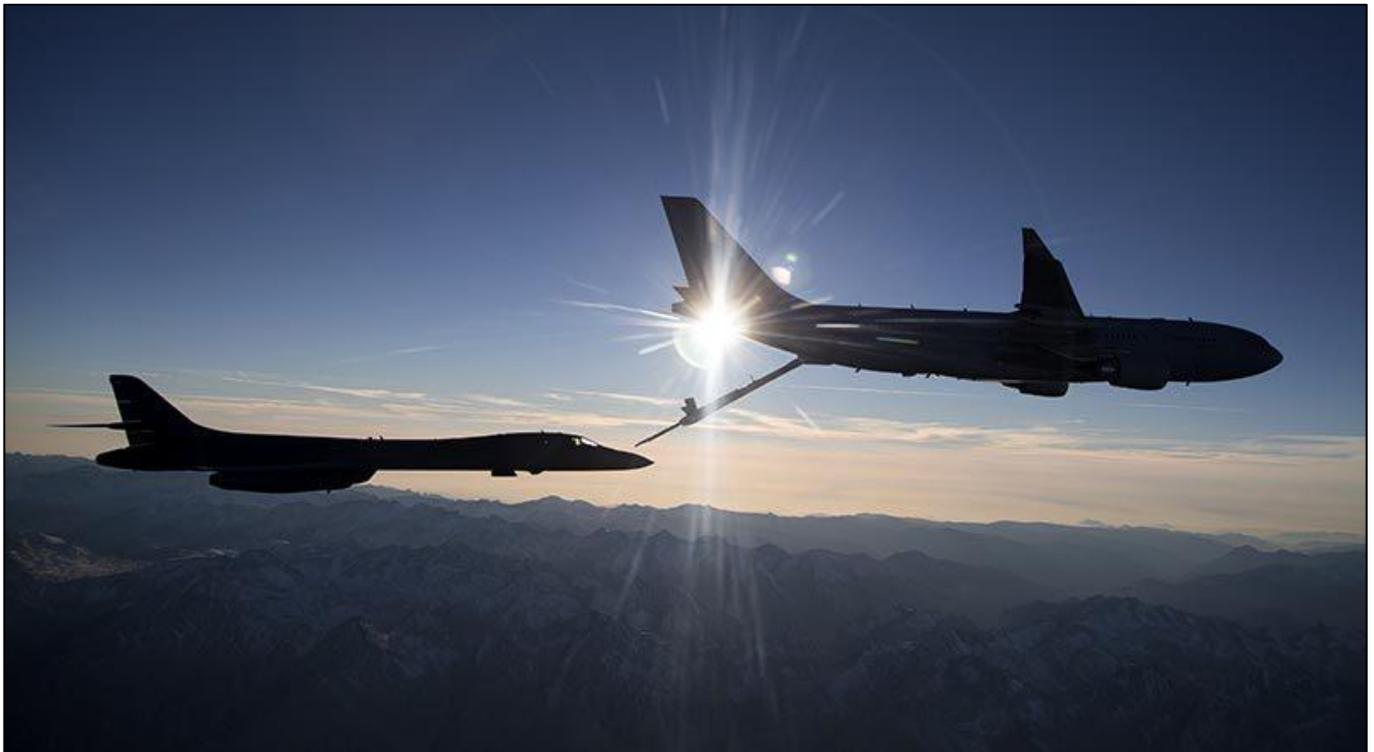
The test team, led by the RAAF's Aircraft Research and Development Unit and the USAF's 418th Flight Test Squadron, examined all parameters of the air-to-air refuelling procedures between the two aircraft, with a total of 185 dry contacts and 16 wet contacts (where fuel was transferred) being conducted.
