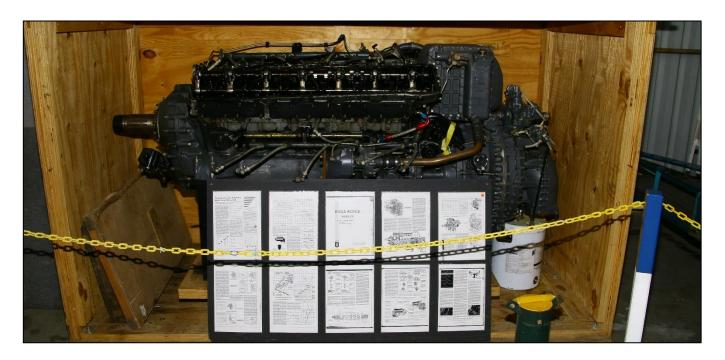
The V-12, 27 litre, Rolls Royce Merlin engine was first run in 1933. The first aircraft to use the engine was the Fairy Battle, then the Hawker Hurricane and then the Supermarine Spitfire, for which it is most closely associated. It also powered the Avro Lancaster. Production of the engine ceased in 1950 after which 160,000 had been built.
