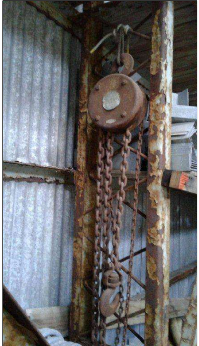
Block and tackle used to remove aircraft engines.
