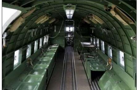
to lift 20-plus passengers and baggage or a 2,750 kg cargo load. Cruising at 260 to 290 kph, the DC-3 has a range of about 2,575 kilometres, land in less than 1,000 km and take off again in less than 300 km. Its low-speed handling and toughness made it the go-to airplane for a myriad of jobs including military special operations.
