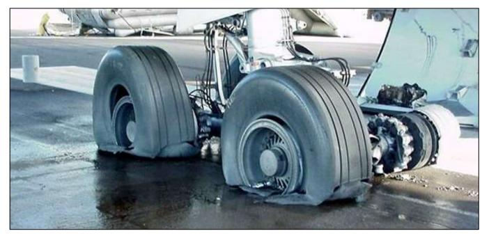
Fourteen passengers and two crew members suffered minor injuries, while two passengers suffered serious injuries during the evacuation of the aircraft. The plane suffered structural damage to the main landing gear and the lower fuselage.
