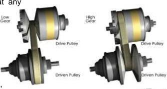
whereas CVTs provide a smooth, rapid increase in maximum power. To some drivers this makes the car feel slower; in fact, a CVT will generally out-accelerate an automatic.
