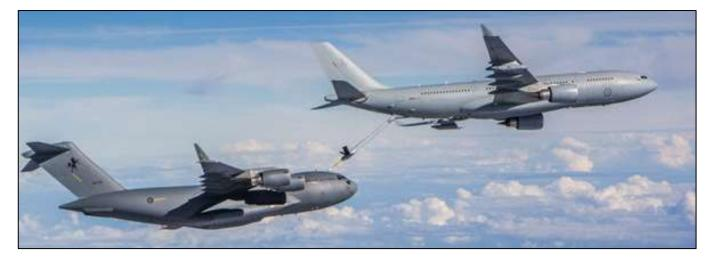
The KC-30A can remain 1800 km from its home base for up to 4 hours to offload 50 tonnes of fuel. It can also carry 270 passengers, and 34 tonnes of freight in pallets and containers.
