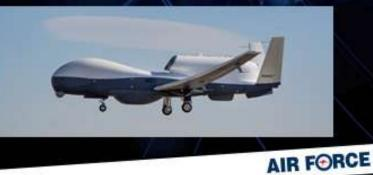
The MQ-4C Triton Unmanned Aircraft System is a High Altitude Long Endurance (HALE) aircraft that will be used from 2020 for maritime patrol and other surveillance roles. Supporting missions up to 24 hours, the Triton is equipped with a sensor suite that provides a 360-degree view of its surroundings for over 2000 nautical miles.
