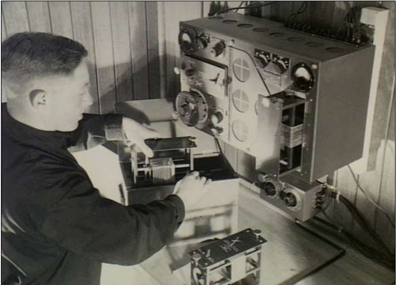
A RAAF Radtech tuning a mobile radio transmitter at the wireless training school at Point Cook. Portable??
