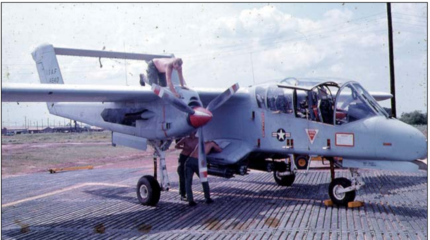
An OV-10 before flight on steel matting at Di An. An improvement on the Dong Tam O-1 revetment.
